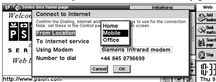
Typical Network login time is 20-30 seconds and typical download time for Psion's home web page ([www.pSION.com](http://www.pSION.com)) is about 2 minutes, this being dependent on having good cellular coverage and high signal level.
