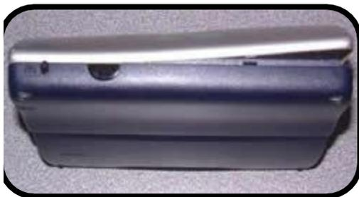
Now you need to be a little careful. The other side of the rear casing hinge does not have a removable pin so do not separate the top and bottom halves too much. There are two small clips holding the two halves as well as this pin. Gently prise the two apart - this is easier to do with the top and bottom halves closed together. Remove the first clip.....
