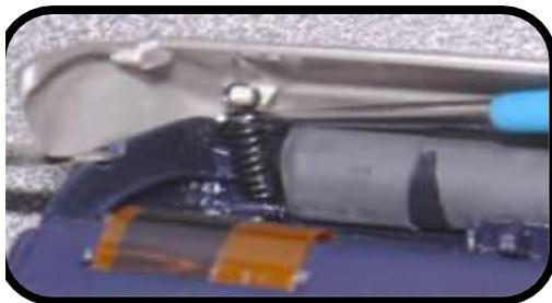
Use the spring hook or similar to remove the top loop of the spring from the small plastic hook in the rear casing. Leave the bottom of the spring attached to the bottom casing. Repeat for the other side.
