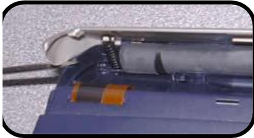
Option 1: The battery pack can be removed from here by holding the rear case open and following the battery removal sections below - I DO NOT RECOMMEND THIS METHOD but it saves the need for a  and some fiddly manoeuvres!
